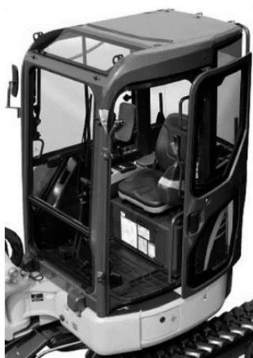
Figure 3–9 Vehicle-based construction machinery with a fall protection structure
