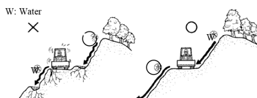
Figure 6-8 Example of slope (nori men) drainage (norimen haisui)
